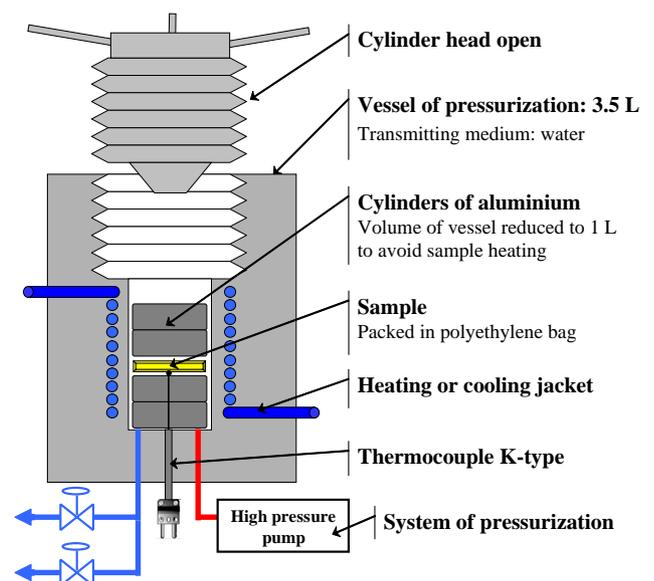
Fig. 1. Schema of the high pressure vessel from ACB pressure systems.
