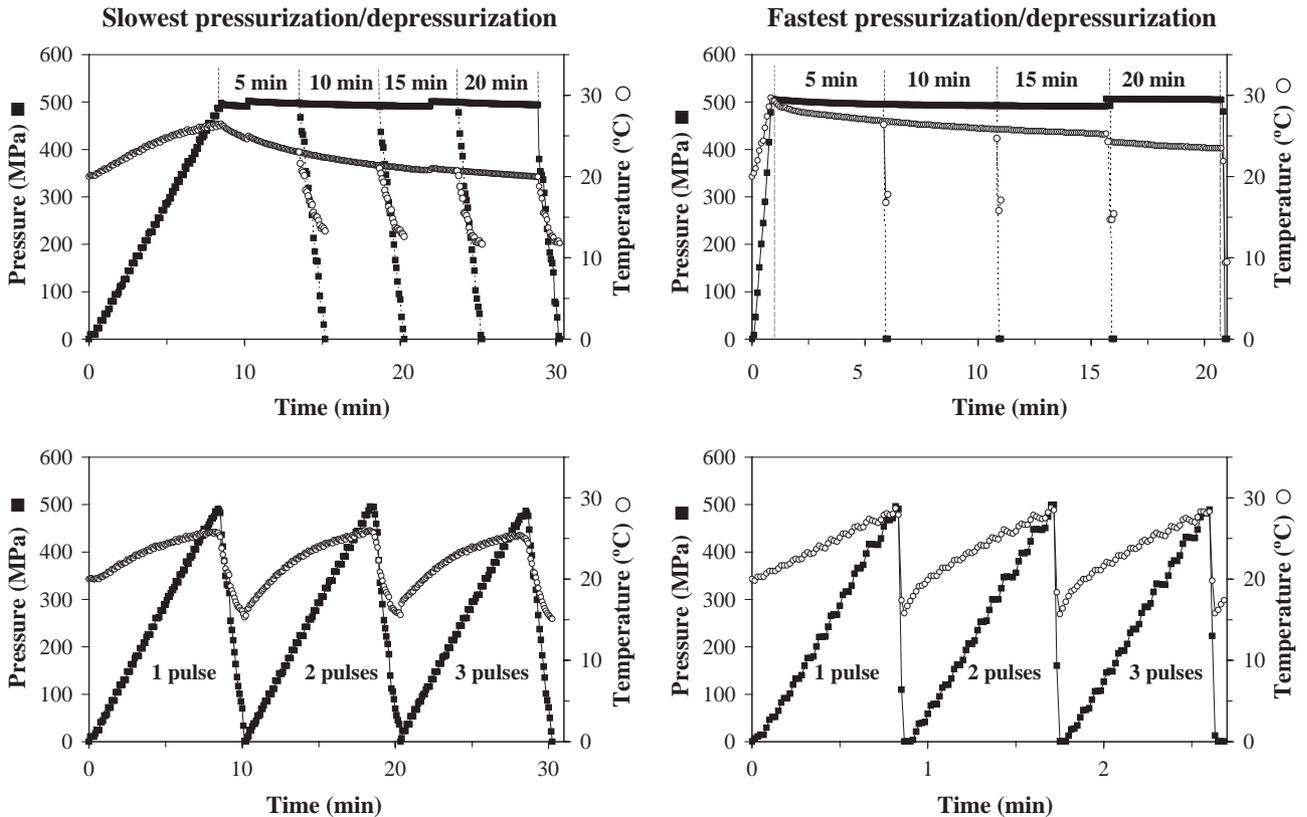
Fig. 2. Temperature and pressure for 500 MPa processing, with the slowest and fastest parameters of pressurization/depressurization on pulse series (1, 2 and 3) and holding time (5, 10, 15, 20 min), ■ pressure in the vessel, ○ temperature near the sample. Each figure is composed by the combination of all the possible treatment applied in the same pressure conditions.
